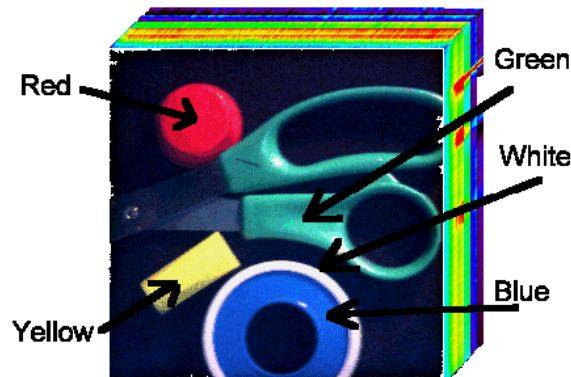
Figure 1. A stack of 32 images of several colored common objects grabbed with OKSI's LCTF camera from 400 to 710 nm.
