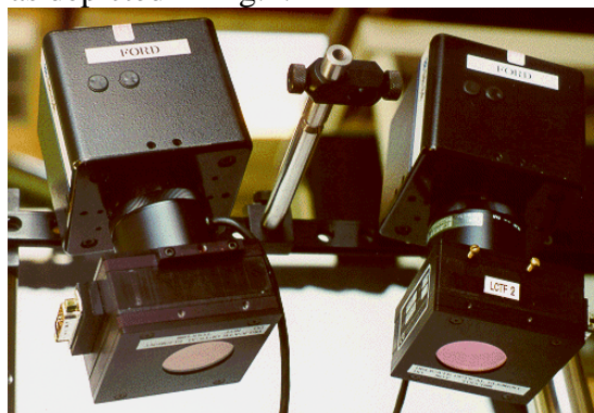
Figure 8. A stereo imaging spectrometer system.
