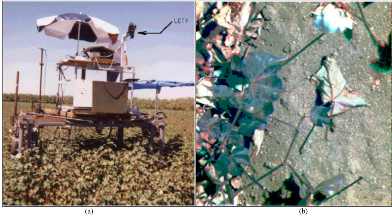
Figure 14. (a) OKSI's LCTF system in precision agriculture ground truth validation produces images such as in (b) showing spectral details of plant canopy and soil that allow measuring spatial variability in properties in support of canopy models and remote sensing observations.
