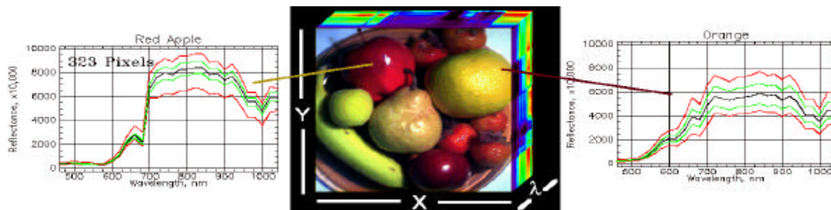
Figure 1. Image cube obtained with a liquid crystal tunable filter; providing high spatial resolution of spectral features.
