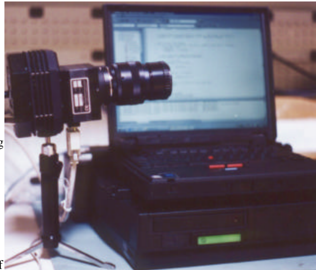
Figure 9. A portable spectral imaging system uses a laptop with a docking station to accommodate up to 3 PCI boards for frame capture, additional serial card, and an ethernet card.
