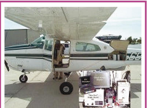
Airborne Sensors provide a georeferenced image map of a field allowing very accurate mapping of crop health stress conditions
