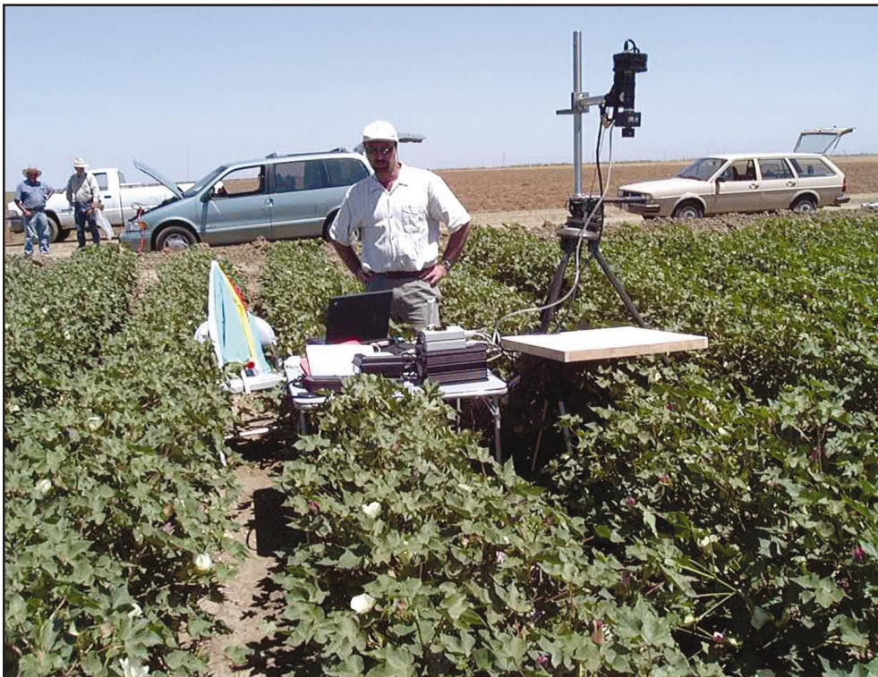
The Sheely farm is one of several sites testing precision agriculture techniques as part of the Ag20/20 program. Here, Gordon Scriven of Opto-Knowledge Systems Inc. collects hyperspectral data on the ground that will be used to validate airborne measurements of the cotton fields.
