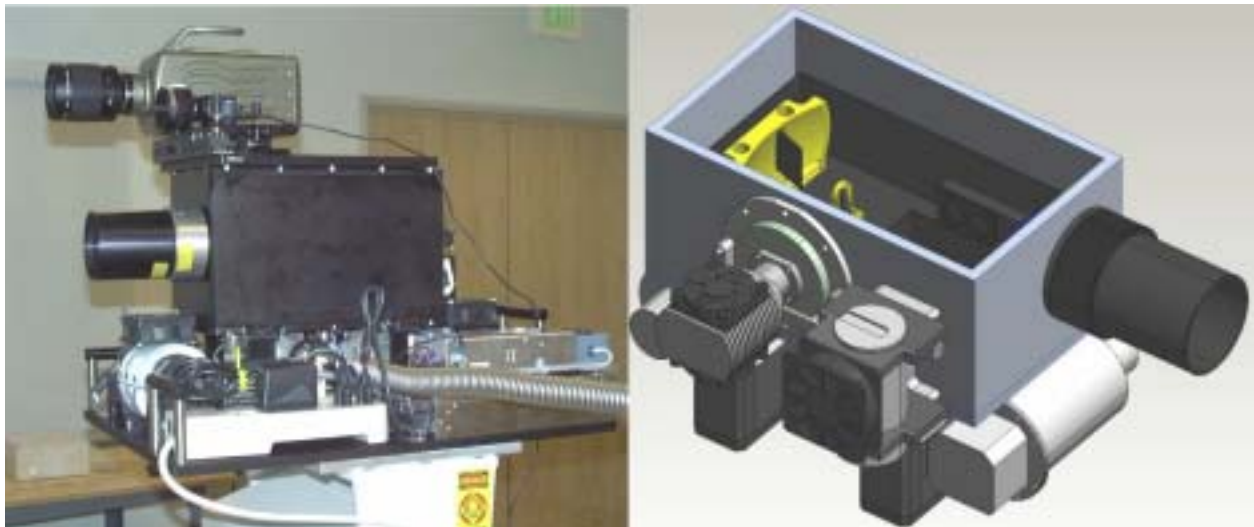
Figure 7. MWIR 4D-IS: actual sensor (left) with a bore-sighted Phantom and wide FOV tracking cameras on top, and a 3D CAD with the radiation shield removed (right). The sensor is designed for airborne operations and is cooled with Stirling cryo-coolers.
