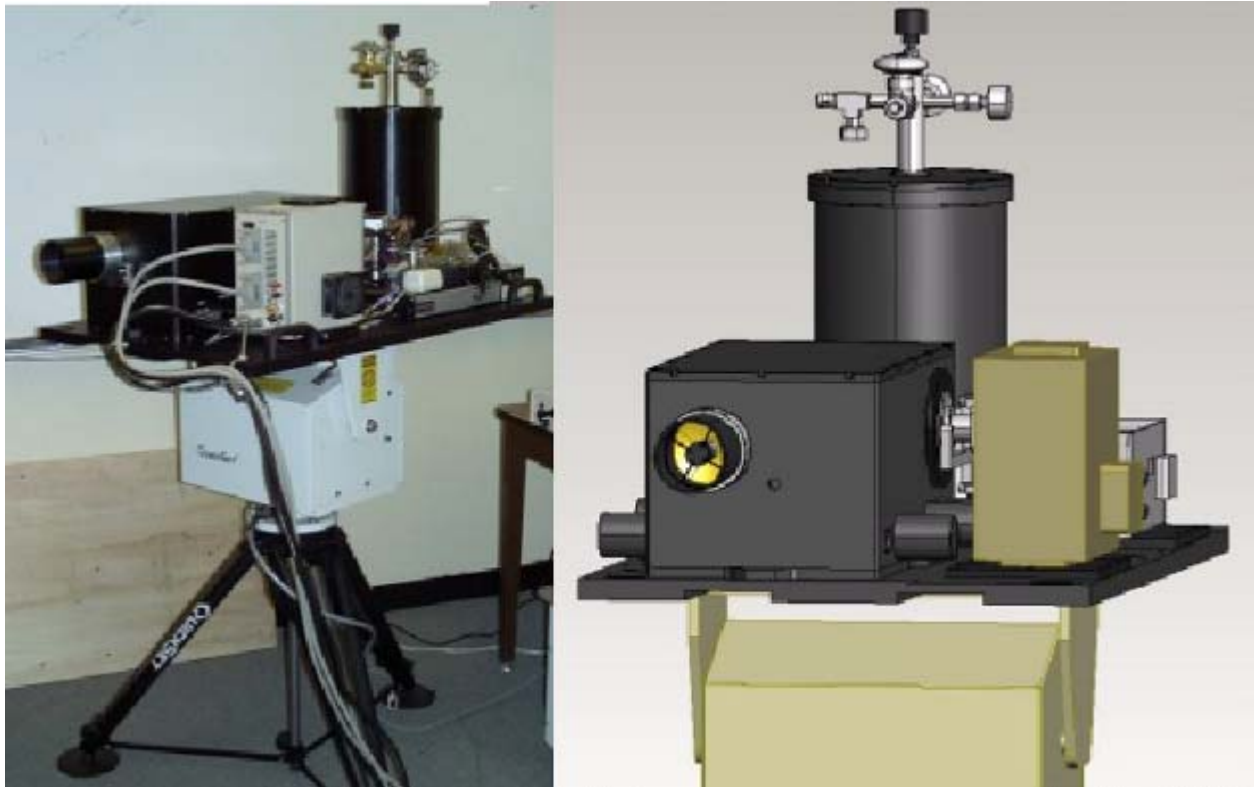
Figure 6. MW/LWIR 4D-IS sensor: actual system (left), 3D CAD model (right), showing the maintenance LN2 dewar in the back, which allows the sensor to run for several hours without connection to a large LN2 tank. The sensor is mounted on a custom designed plate that fits on standard KTM tracker mounts.
