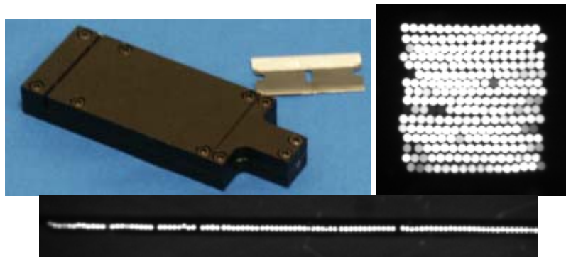
Figure 5. Chalcogenide rigid reformatter (top left), showing the 2D and partial 1D ends.
