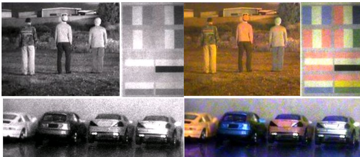
Fig. 1. Monochrome and color low-light-level imagery. The images illustrate the additional information that is available with the inclusion of color.
