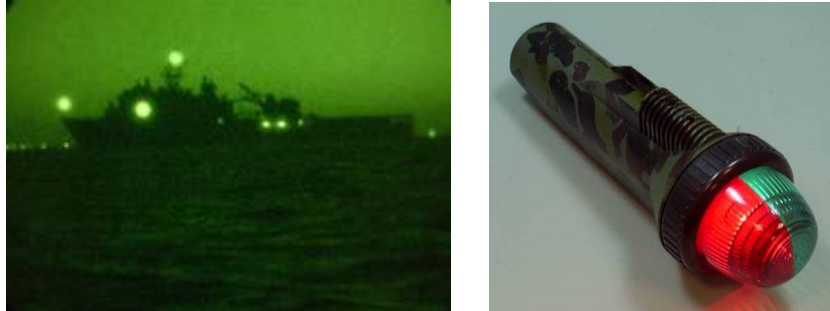
Figure 12. (Right) Image of ship with navigation lights taken with a monochrome low-light-level camera. (Left) Example light used to test TCNV technology.
